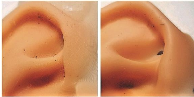
Fig. 21. Surface quality of the prosthesis printed with the form 2 (left) and Elegoo Mars (right) (De-Rossi-Estrada et al, 2020).
