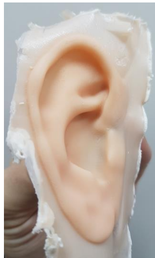
Fig. 14. Silicone model with flash before post-processing. (De-Rossi-Estrada et al, 2020).
